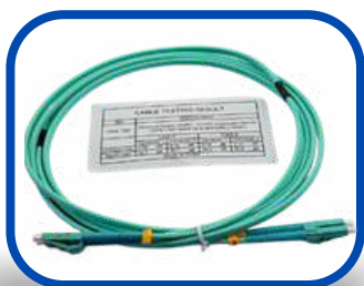
LC/LC/UPC,OM4, Duplex,LSZH,3.0 mm,2mtr
